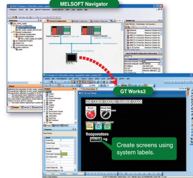
Configure a system combining GOT and PLCs and set up GOT I/F and communication drivers using MELSOFT Navigator, the system management software for the FA integrated engineering software package MELSOFT iQ Works.
