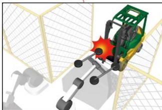
Dangerous when loading materials without noticing the production line in operation.
