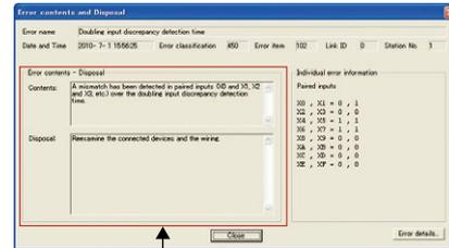
CC-Link Safety remote I/O errors can be easily displayed
