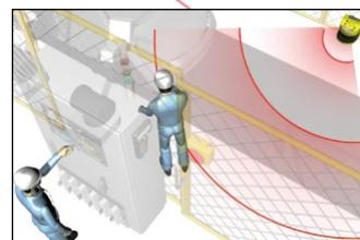
By detecting laser scanner signals, startup is interlocked when an operator enters an exclusion zone, even if the operator is obscured from view.
