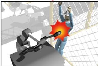
An operator loading materials can be caught between a robot area and a fence.
