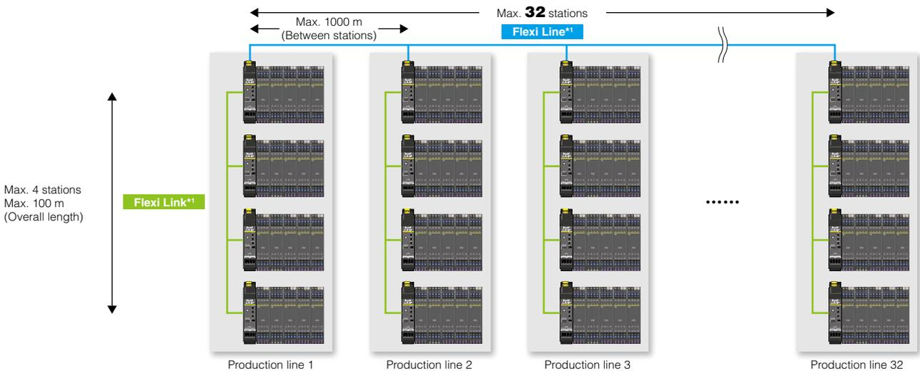
\*1. Flexi Line is supported by WS0-CPU3 only and Flexi Link is supported by WS0-CPU1 and WS0-CPU3 only. For details about network specifications, refer to page 11.
