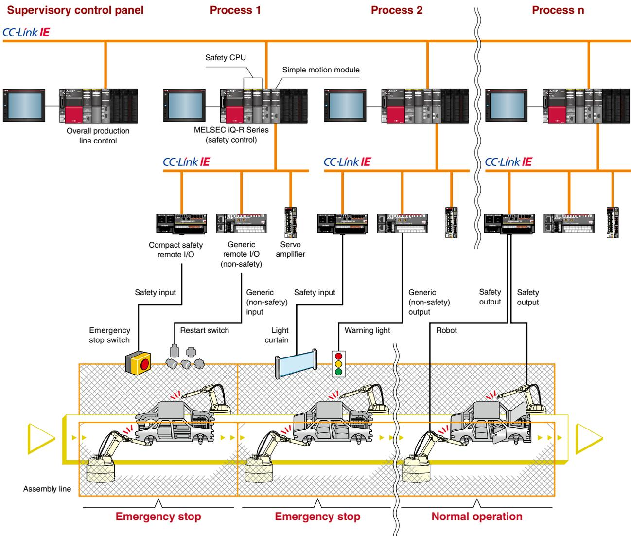
Error occurs at Process 2. Stations at Process 1 and Process 2 are made to stop with an emergency. Station at Process n keeps operation.
