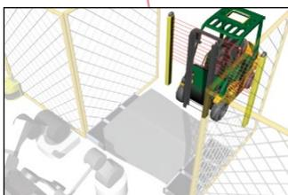
The production line is safely stopped by detecting light curtain signals when an operator enters the exclusion zone.
