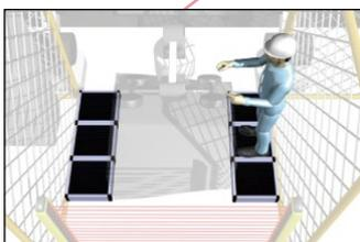
The production line cannot start while an operator is within the area as detected by the safety mat.
