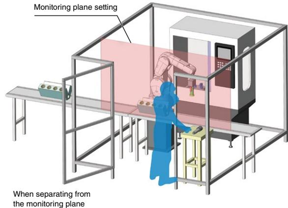
Area sensors secure the safety without safety fence
