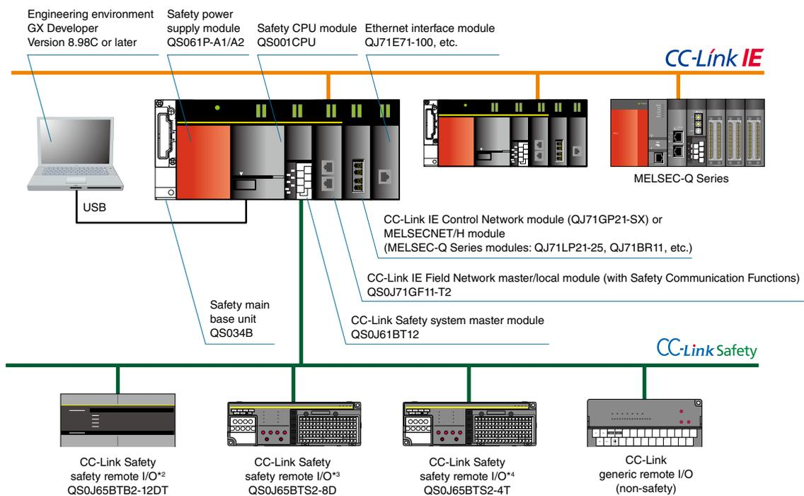
\*2. Number of input points: 8 points (double wiring), No. of output points: 4 points (source + sink type)
