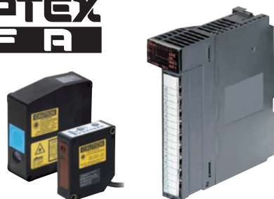
Control unit UQ1 series Sensor head CD5 series (high accuracy type, measurement range : 30 \pm 5/85 \pm 20/150 \pm 40/350 \pm 100/500 \pm 200/2000 \pm 500 mm), CD33 series (compact type, measurement range : 30 \pm 4/50 \pm 10/85 \pm 20/120 \pm 60/250 \pm 150 mm)
