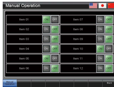
Manual operation (6 patterns) Executes ON/OFF operations of signals (bit devices)
