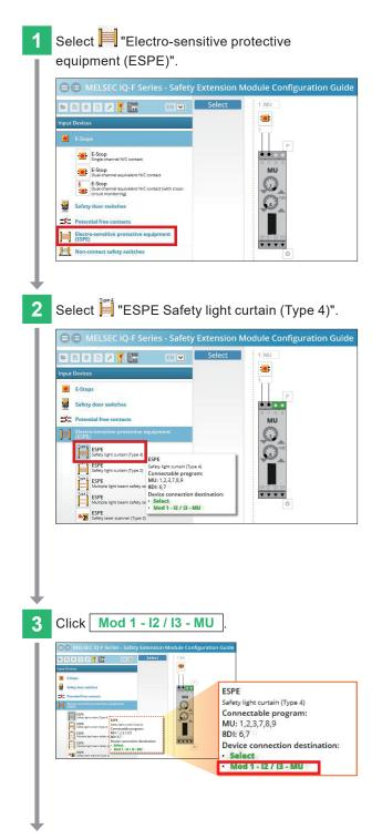
The connection configuration of the emergency 4 stop pushbutton and safety light curtain to the safety main module is displayed.
