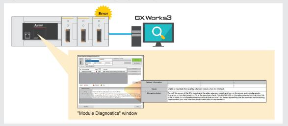
Information such as safety device settings and input/output status can be checked in the buffer memory, reducing the recovery time.
