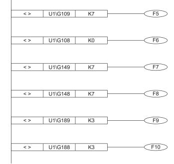
If the FUNCTION rotary switch of the safety main module is not set to '7', the annunciator number 5 turns ON.
