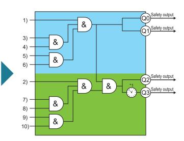
\*1: This is an off delay time. The factory default setting of the rotary switch is 0 second.
