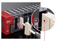
Matching marks on the slot and the cable
