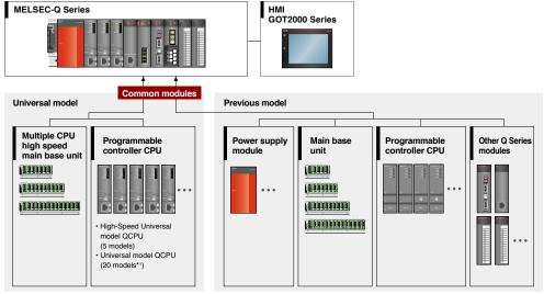
\*1. The Q00UJCPU is all-in-one type, with integrated power supply, 5-slot base unit, and CPU.
