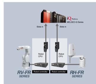
Q Platform makes it possible to structure optimum controllers for various lines.
