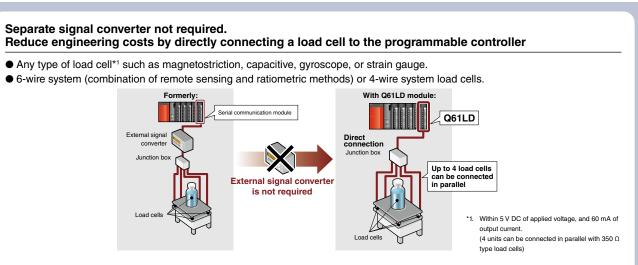
Applications requiring high accuracy can be achieved by connecting the load cell directly to the programmable controller.
