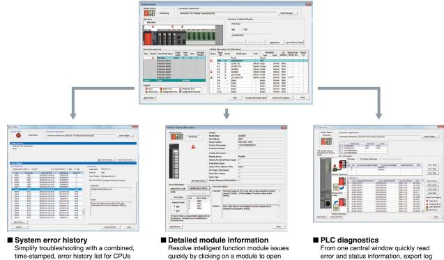
Resolve intelligent function module issues quickly by clicking on a module to open this function. All of the information relevant to the module is displayed here including error codes, their description, and possible solutions. From one central window quickly read error and status information, export log files to CSV, perform remote CPU operations like reset, stop, CPU memory format. and more.
