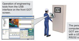
The personal computer and the GOT are connected with a USB cable or RS232 cable
