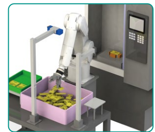
Picking from a large pallet (Fixed camera)
