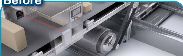
[Current] Inverter + Induction motor (+proximity sensor)
