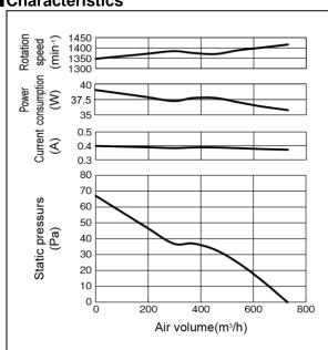
XThe air volume was measured using the orifice chamber method.
