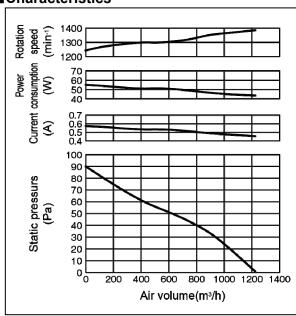
% The air volume was measured using the orifice chamber method.
