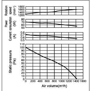
% The air volume was measured using the orifice chamber method.
