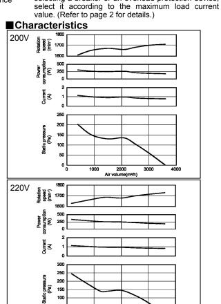
2000 Air volume(m³/h) 1000 ※The air volume was measured using the orifice chamber method
