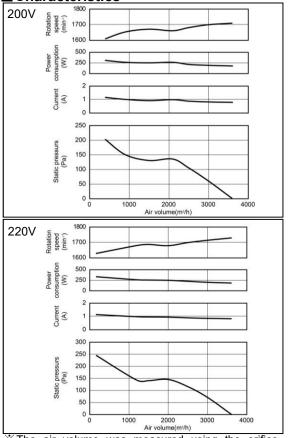
The air volume was measured using the orifice chamber method.
