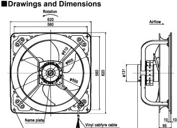
4conductors AWG18 Effective length about 1m
